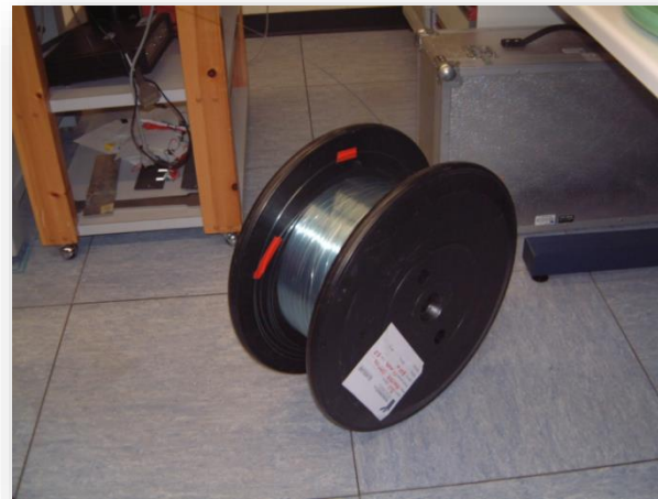
1 km long, 1 mm diameter cable
