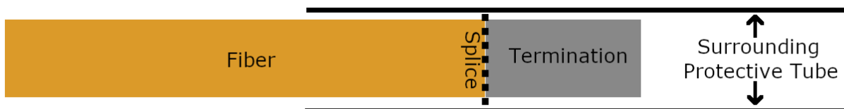
Figure 9-1: Illustration of the termination end of a Luna fiber sensor
