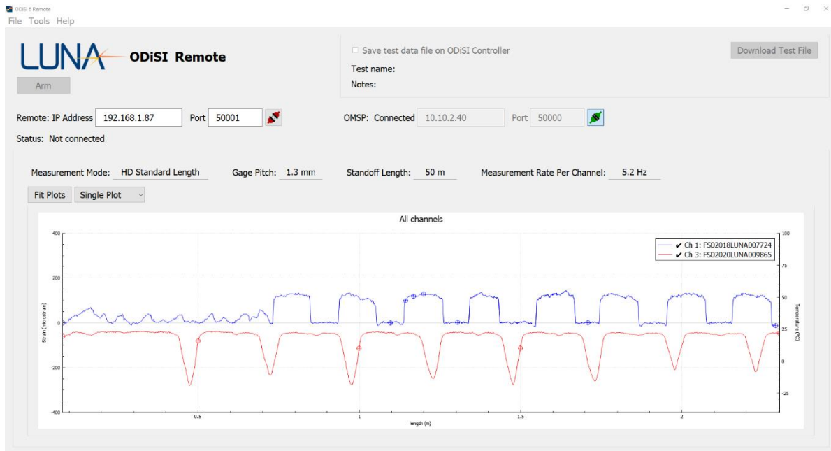
Figure 7-2: ODiSI Remote Sensor Plot
