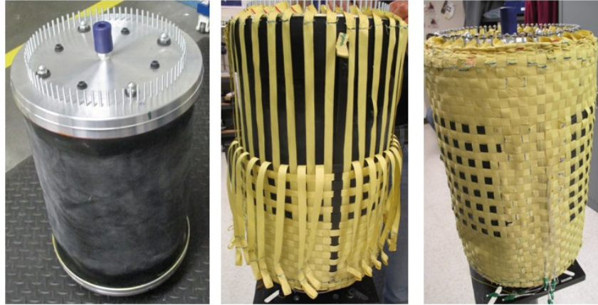
Figure 5: Fabricated inflatable test article prototype, (left) Bladder bonded to endcaps, (center) Weaving process, (right) Finished inflatable structure, black straps are instrumented with fiber optic sensors.
