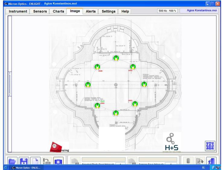
Example software interface showing multiple points of strain, temperature, and acceleration sensors all indicating "green" status
