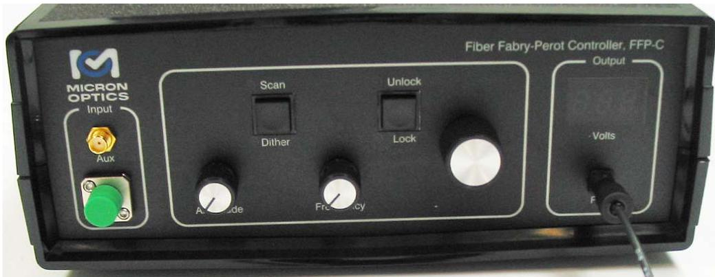
Figure 3. FFP-C front panel.
