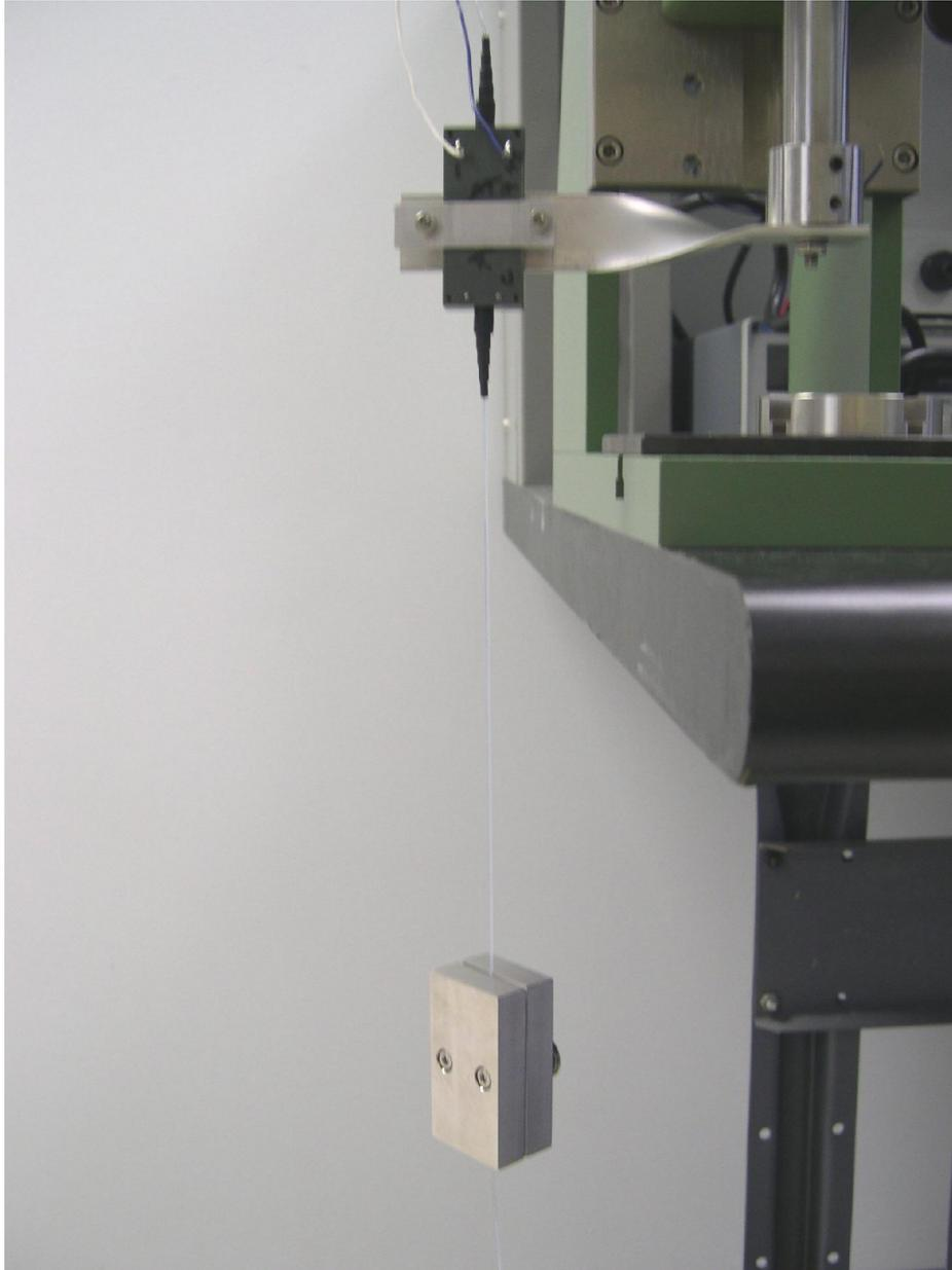
Figure 18: Cable Retention Test Setup
