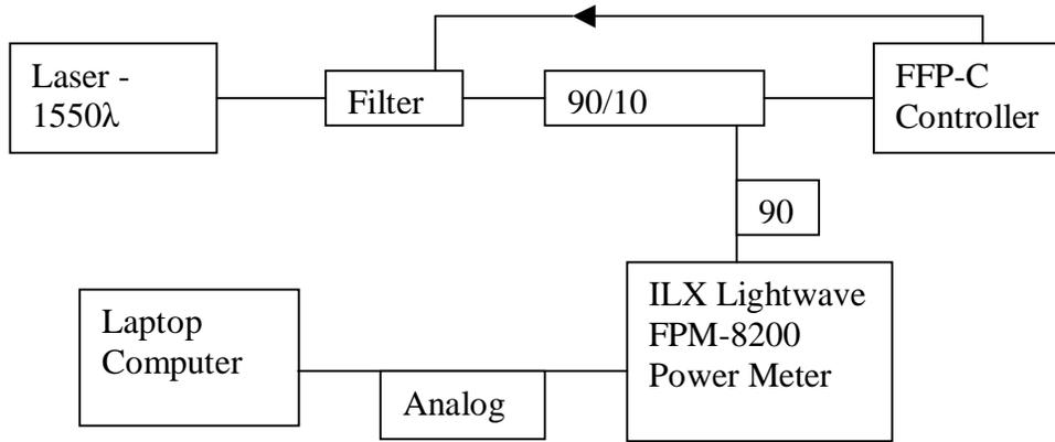
Figure 7: Office Vibration Test Setup
