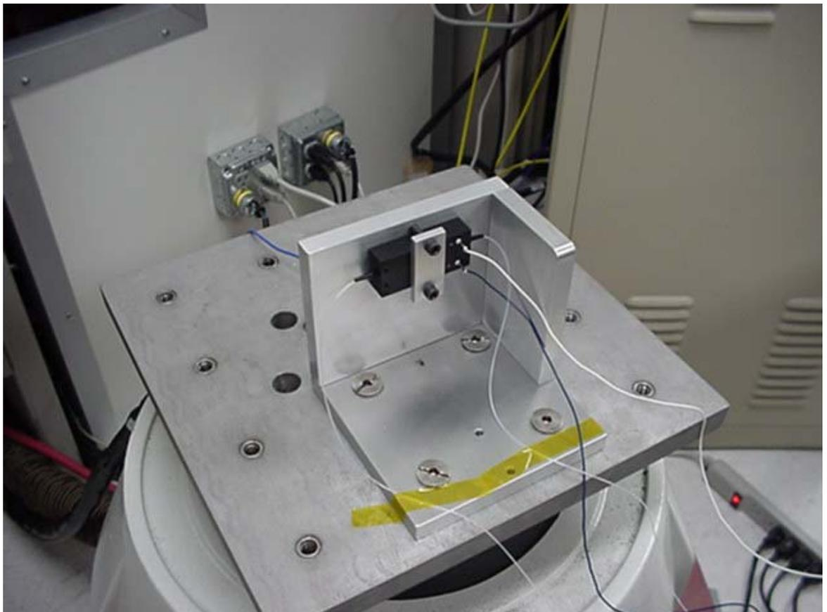
Figure 1: Device and Fixture mounted on vibration table
