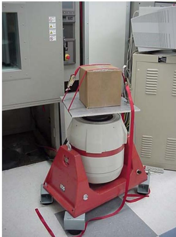
Figure 1: DUT in Shipping Box Strapped to Vibration Table
