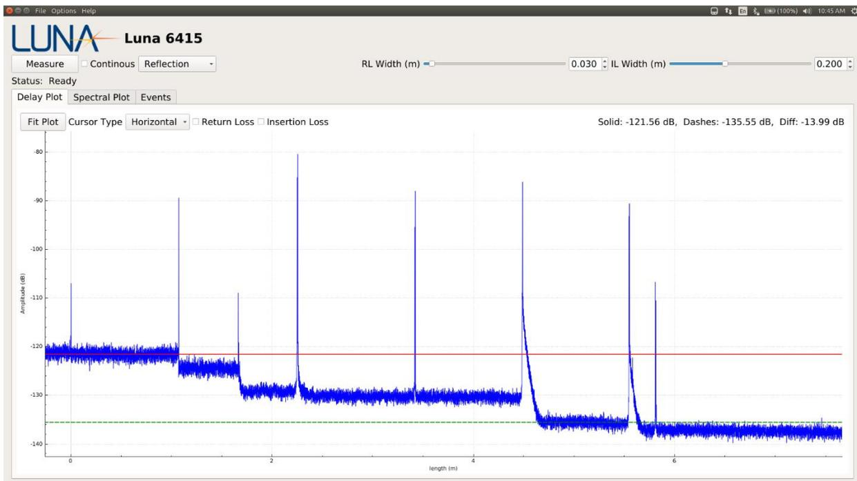
Figure 6-1 Reflection measurement of a fiber array
