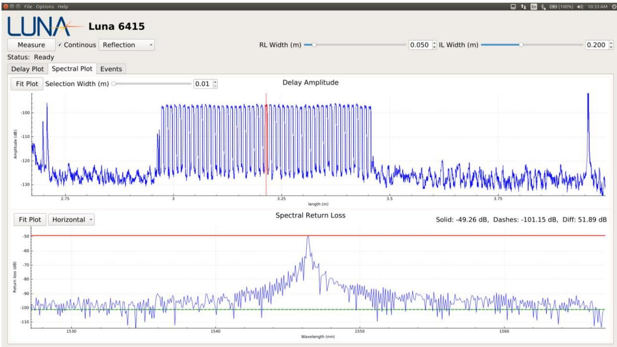
Figure 6-2 Spectral amplitude response plot showing the spectral amplitude of a single FBG
