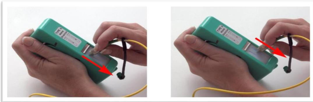
Figure 7-4 - Cleaning the Connector on the Tape
