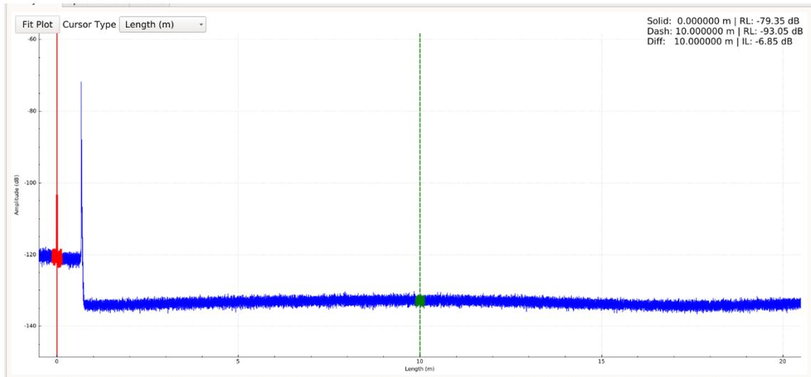
Figure 31 RL measurement using 0.25m RL integration width
