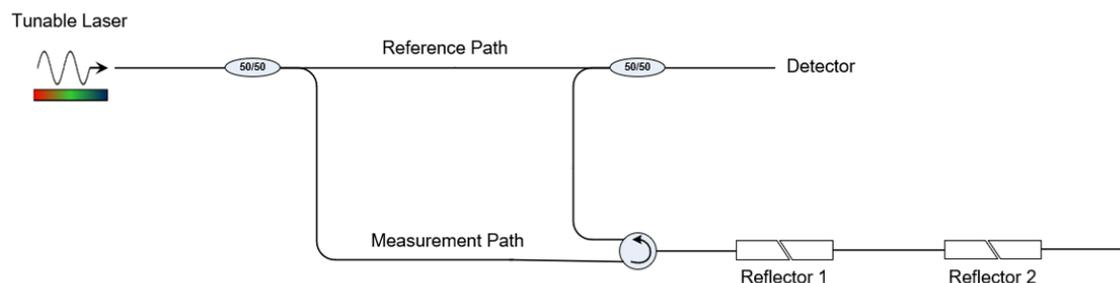
Figure 29 Basic OFDR Optical Network with two partial reflectors (connectors)
