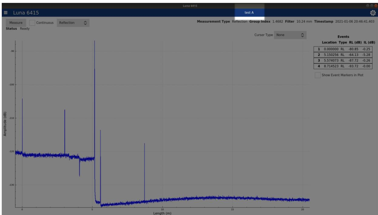
Figure 19 Test name is displayed on the top of screen after a test file is loaded
