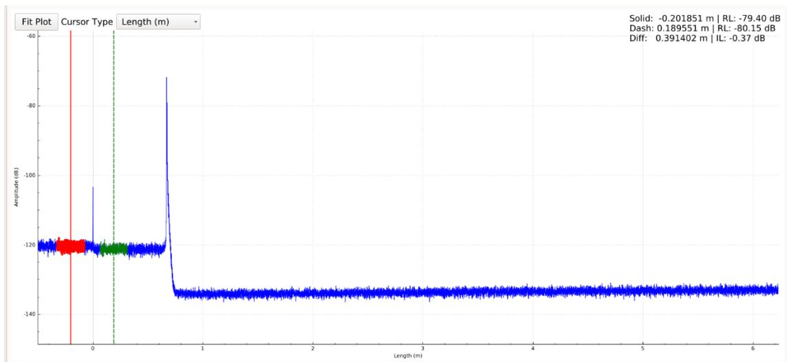
Figure 33 Insertion loss measurement shown across an APC fiber connector. (IL is shown in upper right corner)
