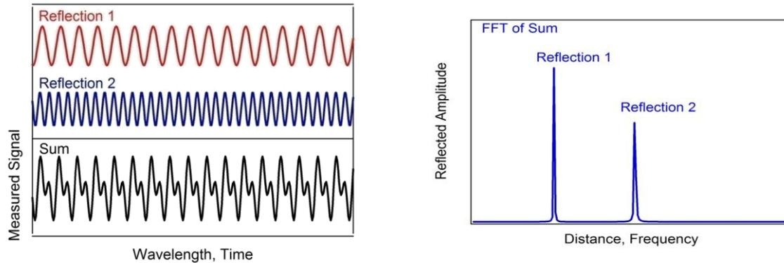
Figure 30 Resulting interference pattern from two reflectors at different locations
