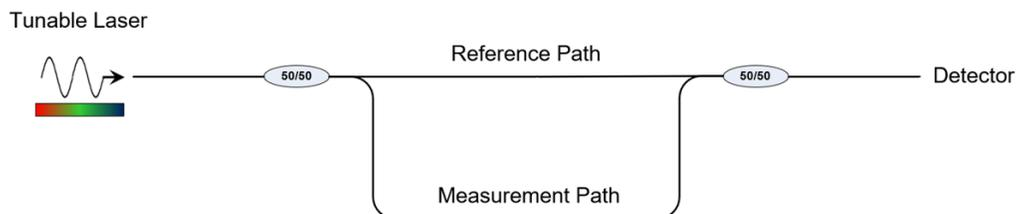
Figure 27 Fiber Optic Interferometer Network
