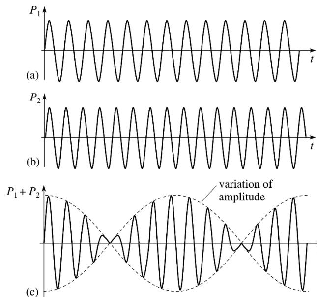
Figure 26 Interference pattern from two waves of differing frequency
