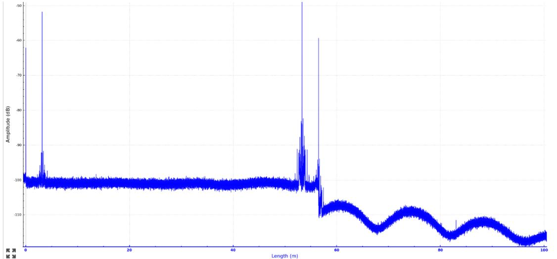
Figure 12 Example of 57m fiber chain viewed in the 100m measurement mode (default 67m focus)
