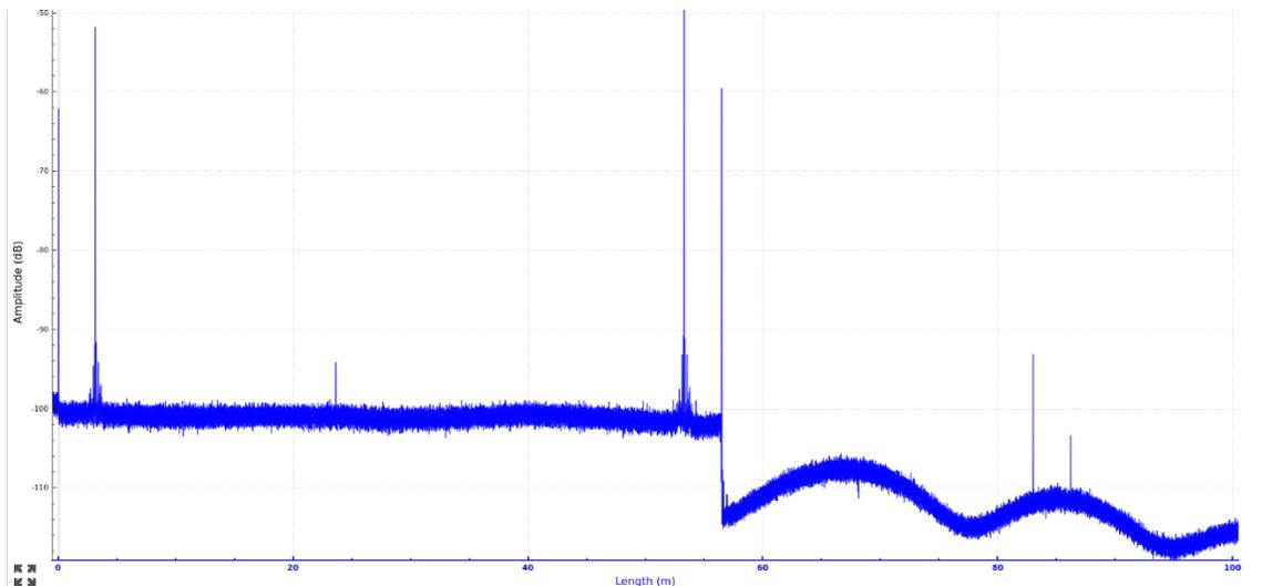
Figure 13 Example of same 57m fiber chain viewed in the 100m measurement mode (57m focus)
