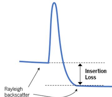
Figure 6. Measuring insertion loss (IL) using backscatter levels
