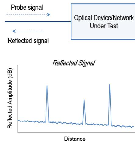
Figure 2. Measurement of return loss using reflectometry
