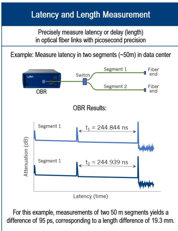
Figure 11. Example measurement of latency/length of optical fiber
