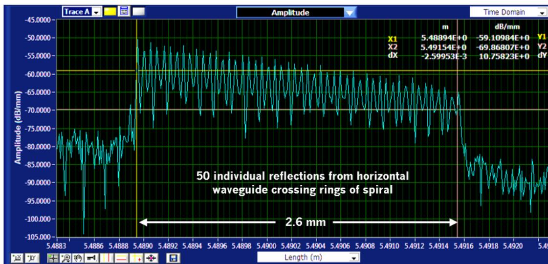
Figure 10. OBR scan of silicon photonics waveguide device
