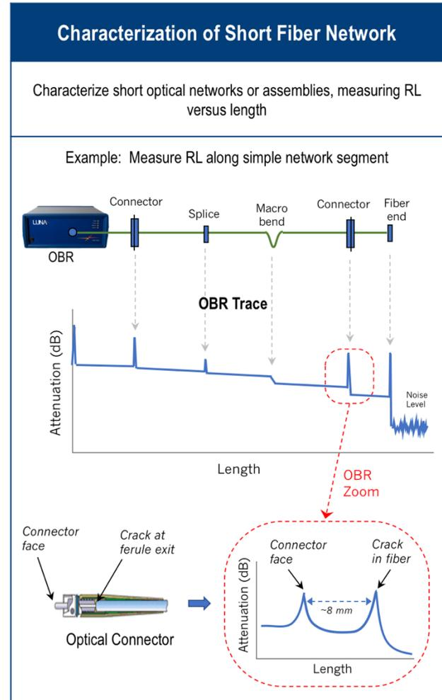
Figure 8. Example OBR measurement of short fiber network
