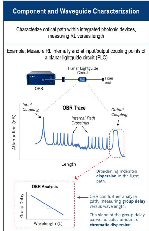
Figure 9. Example OBR measurement of PIC component
