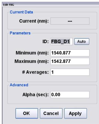
Note that the default wavelength bin width of 2nm has been applied to FBG\_D1.
