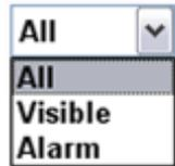
Allows the user to choose among displaying "All" sensors, only sensors which have been declared as "Visible", or only sensors that are presently or have recently been in an alarm state without a reset action applied.
