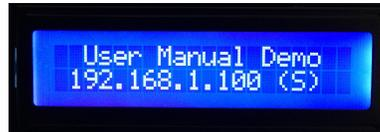
When on the IP settings screen at 15 second long press will cause the instrument to return to its factory default IP settings of address: 10.0.0.55, netmask 255.255.255.0.
