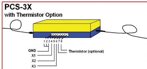
Fig. 2(b) Wiring diagram for PCS-3X and MPC-3X with thermistor option.
