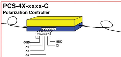
Fig. 2(c) Wiring diagram of PCS-4X-XXXX-C and MPC-4X model for polarization control applications. Pin 8 and pins 1-3 are connected internally.
