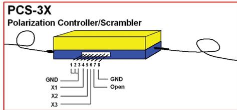
Fig. 2(a) Wiring diagram of PCS-3X and MPC-3X as polarization controller and/or scrambler. Pin 8 and pins 1-3 are connected internally.
