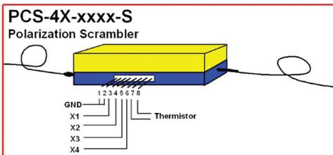
Fig. 2(d) Wiring diagram of PCS-4X-XXXX-S model for polarization scrambling.
