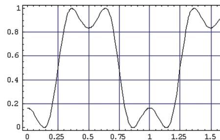
Fig. 3 The optical transmission waveform detected from scope under the condition  $V_{pp} = 1.53 V_{\pi}$
