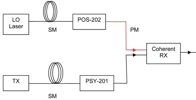
Sample setup for a coherent receiver performance test using a polarization stabilizer (POS-202) and a polarization synthesizer (PSY-201).
