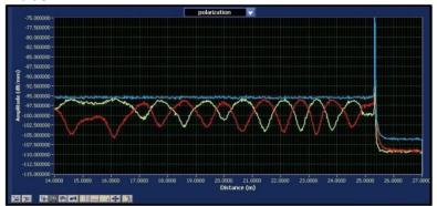
In this case, the period of the white and red traces is equivalent to one half the beat length of the birefringence induced by coiling the fiber (half, because in reflection the light traverses the birefringence twice).
