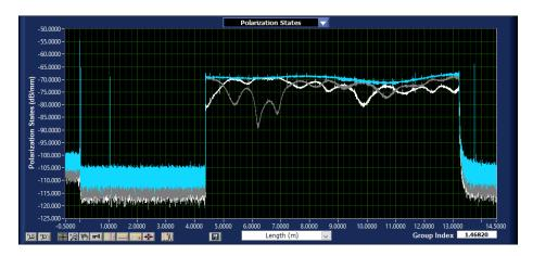
The period of the oscillations of the white and grey traces varies over the length of the grating, from roughly 1.5 to 1 m; so the Beat Length is varies roughly 3 to 2 m. This is likely a consequence of the fiber the FBG is in being coiled up in the module it is housed in.
