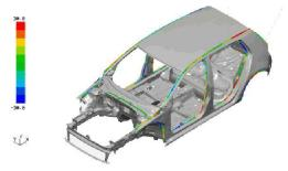
An automotive frame is instrumented with fiber optic strain sensors and tested under load. Color map indicating strain level can be superimposed directly on a CAD model.
