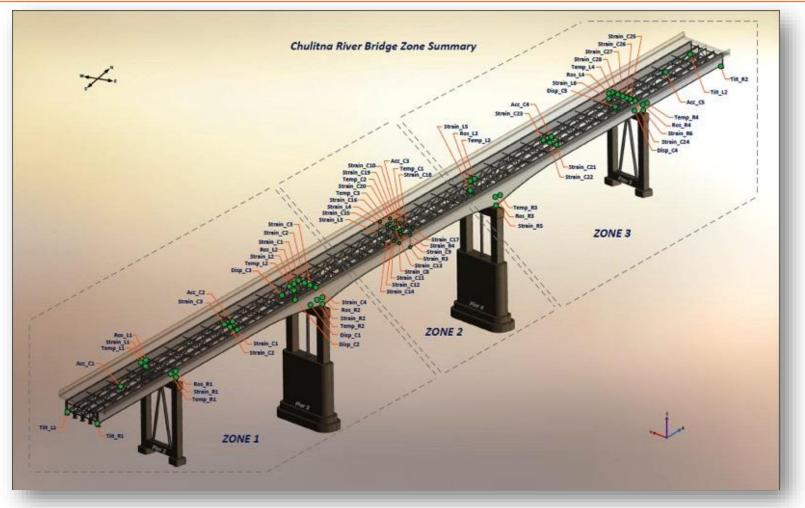
The bridge is divided into three monitoring zones based on the number of sensors in each zone.
