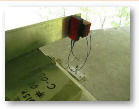
Displacement gages mounted on the rocker bearings monitor movement away from the supports as the bridge expands and contracts in response to the large temperature swings of up to 70°C.
