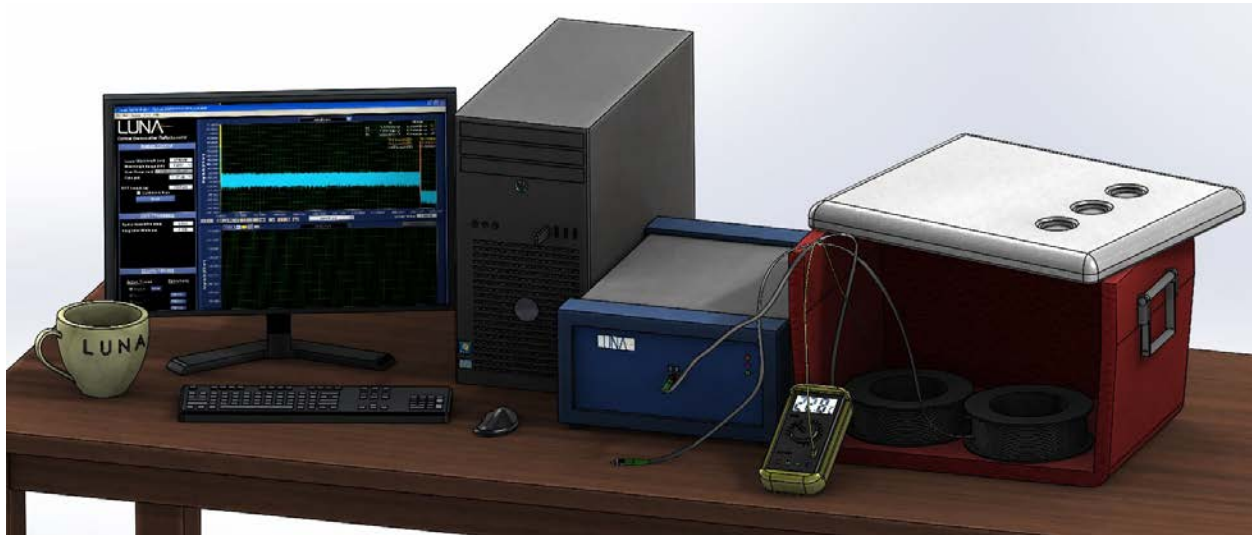
Figure 1: OBR 4600 spool length measurement test setup
