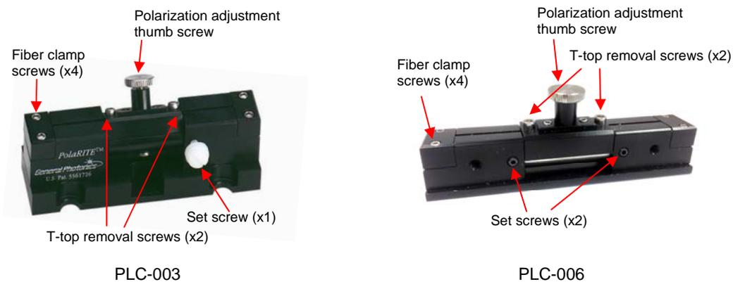
Figure 11 User-adjustable screws on PLC-003/006
