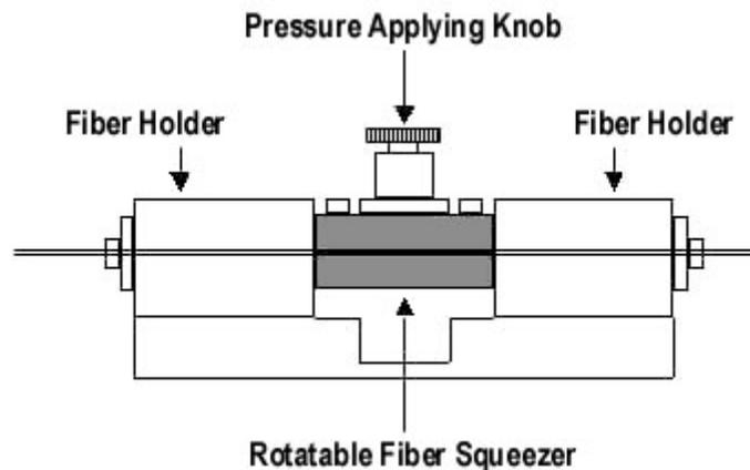
Figure 1 Diagram of manual polarization controller with functional parts labeled
