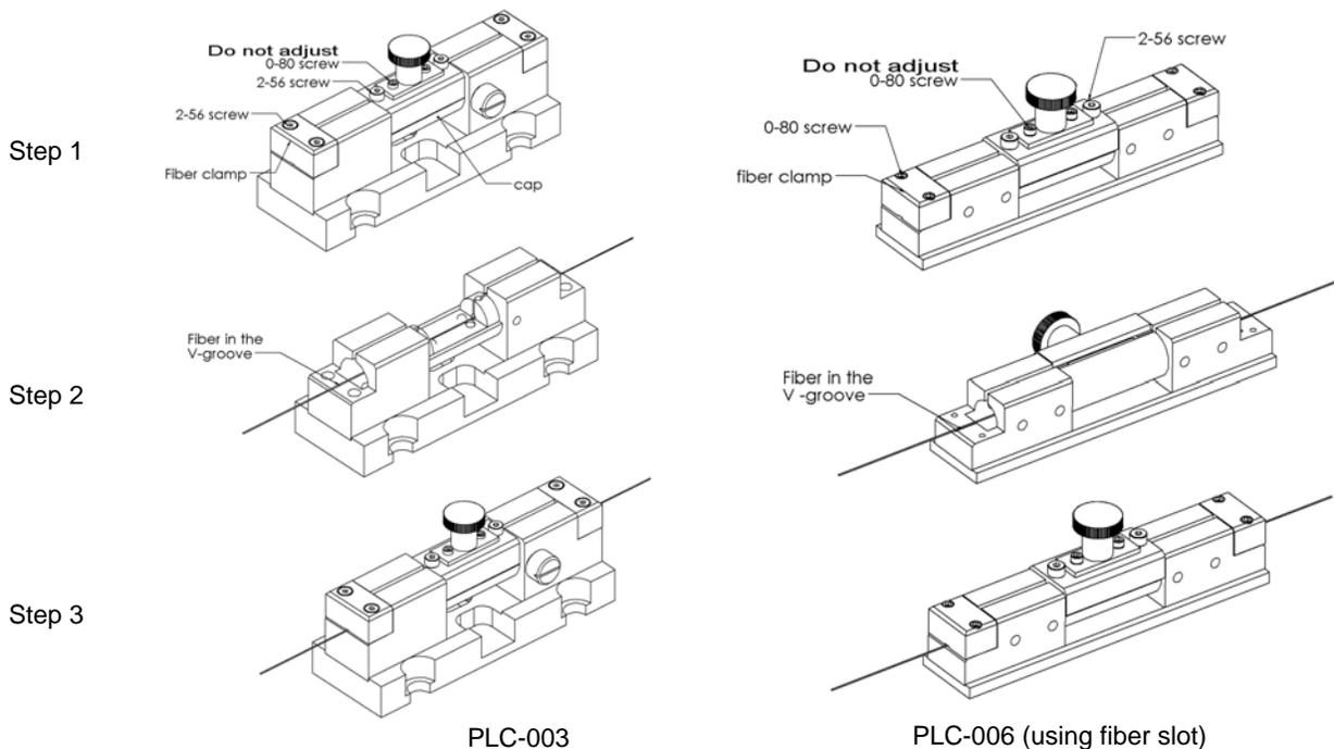
**Figure 2 Fiber placement in drop-in polarization controllers**
