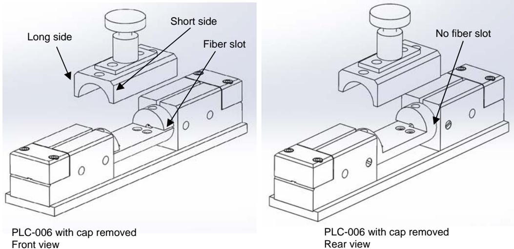
**Figure 3 Center cap alignment for PLC-006**
