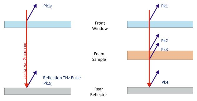
Figure 2 – Sample in External Reference Structure (ERS)
