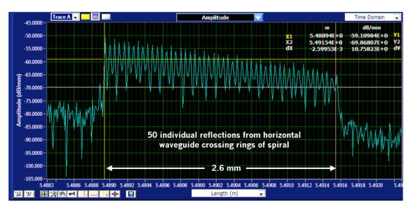
Figure 10. OBR scan of silicon photonics waveguide device
