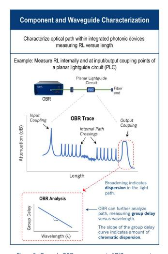
Figure 9. Example OBR measurement of PIC component
