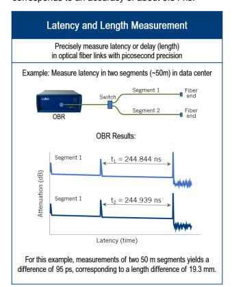
Figure 11. Example measurement of latency/length of optical fiber
