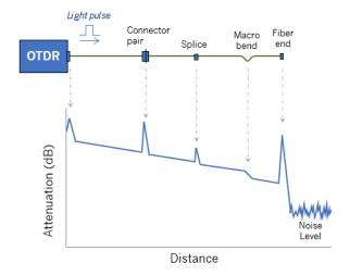
Figure 3. Example OTDR trace for a simple network, mapping loss versus distance
