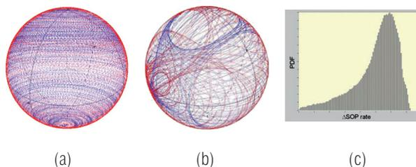
Fig. 3 a) Tornado SOP trace, fixed axis. b) Tornado SOP trace, rotating axis. c) Tornado scrambling SOP rate variation distribution.
